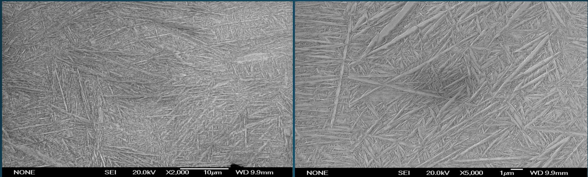
Micrograph X2000 and X5000 3D printed Ti6Al<sub>4</sub>V after etching with 8.8 M H<sub>2</sub>O<sub>2</sub> + 0.1 M HCl at 80°C for 30 min and thermal oxidation at 500 °C
