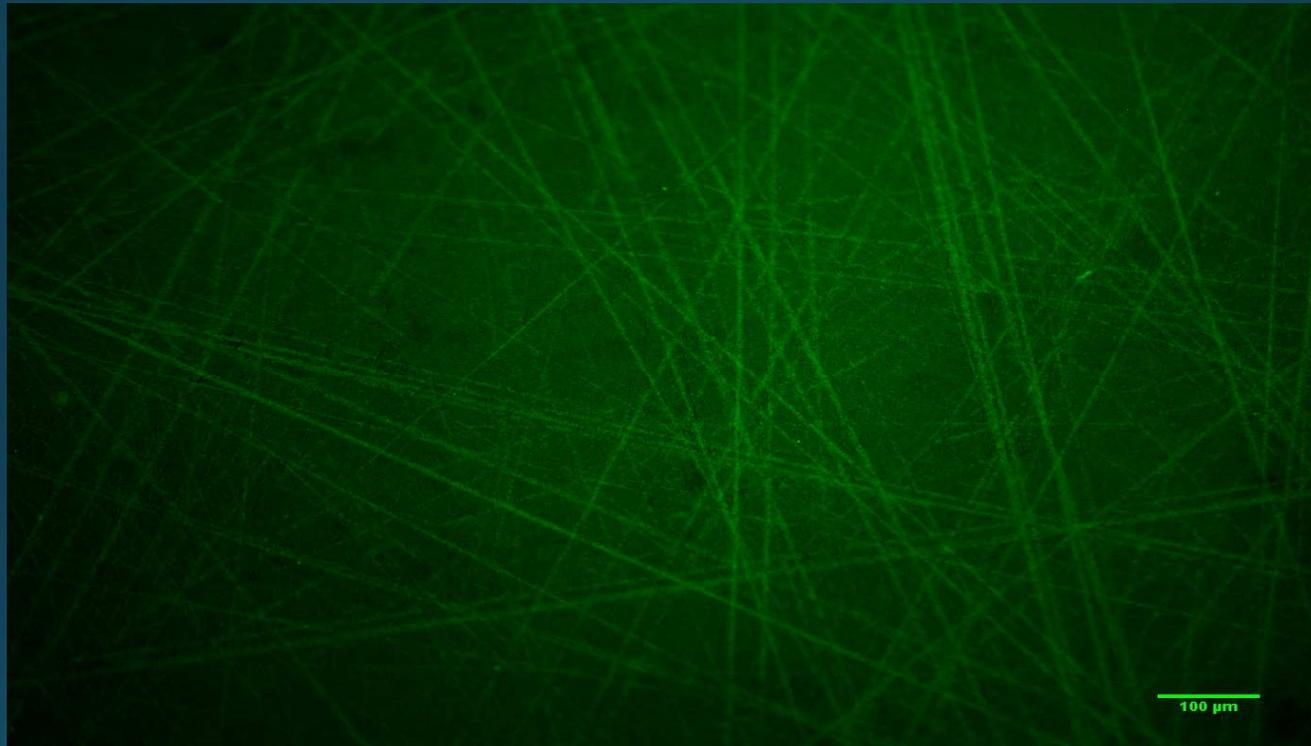
Fluorescence micrograph (100 μm) of 3D printed Ti6Al<sub>4</sub>V (surface A) after dip coating in SBF solution at pH<sub>4</sub> and concentration of 10 μM of labeled peptide aptamers
