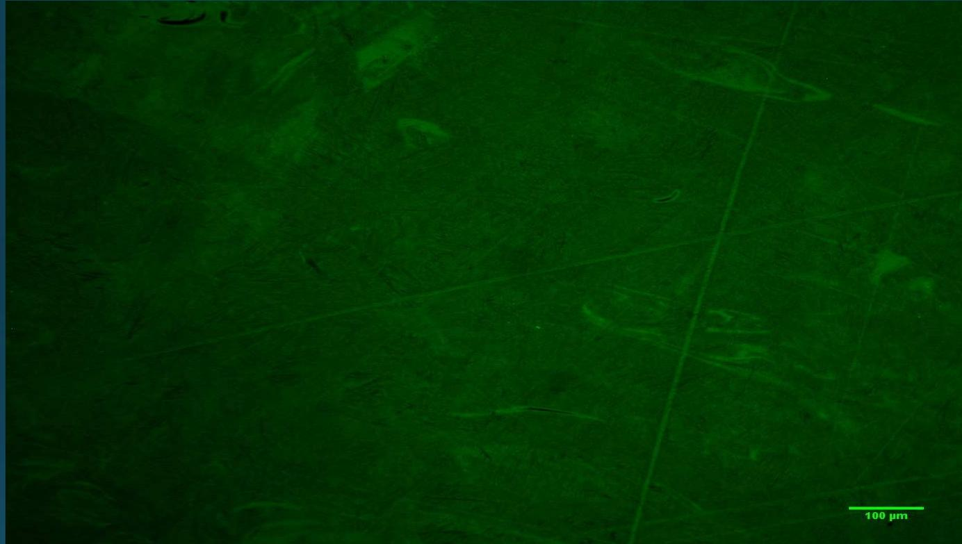
Fluorescence micrograph (100 μm) of 3D printed Ti6Al<sub>4</sub>V (surface B) after dip coating in SBF solution at pH<sub>4</sub> and concentration of 10 μM of labelled peptide aptamer
