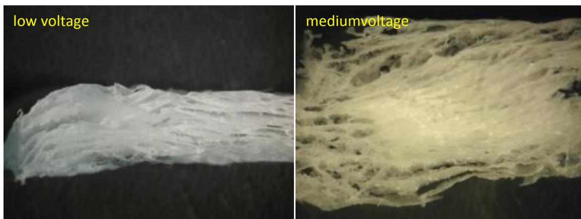
*Figure 1. Stereo zoom microscope images of cross-sections of freeze-dried GG deposits obtained under low (~ 2 V) and medium voltage (~ 5 V)*
