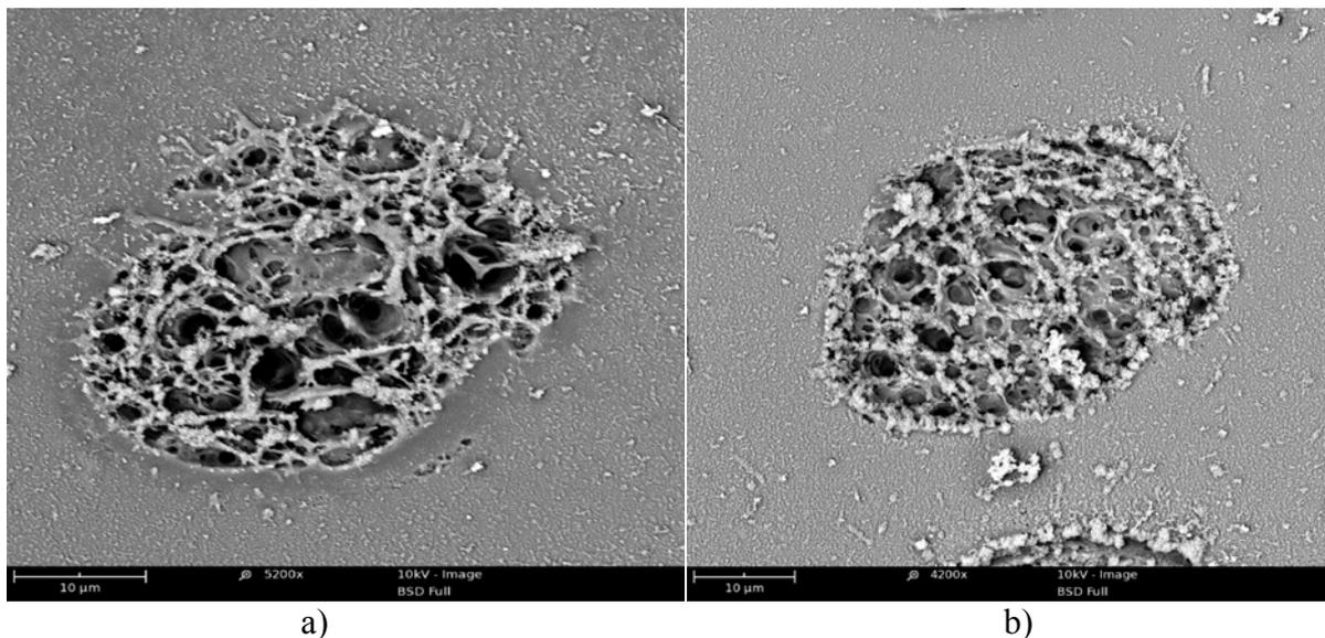
Fig. 3. Chitosan sample treated with different number of pulses, 150 fs, output power 0,1mJ, repetition rate 50 Hz: a) 1 pulse and b) 2 pulses
