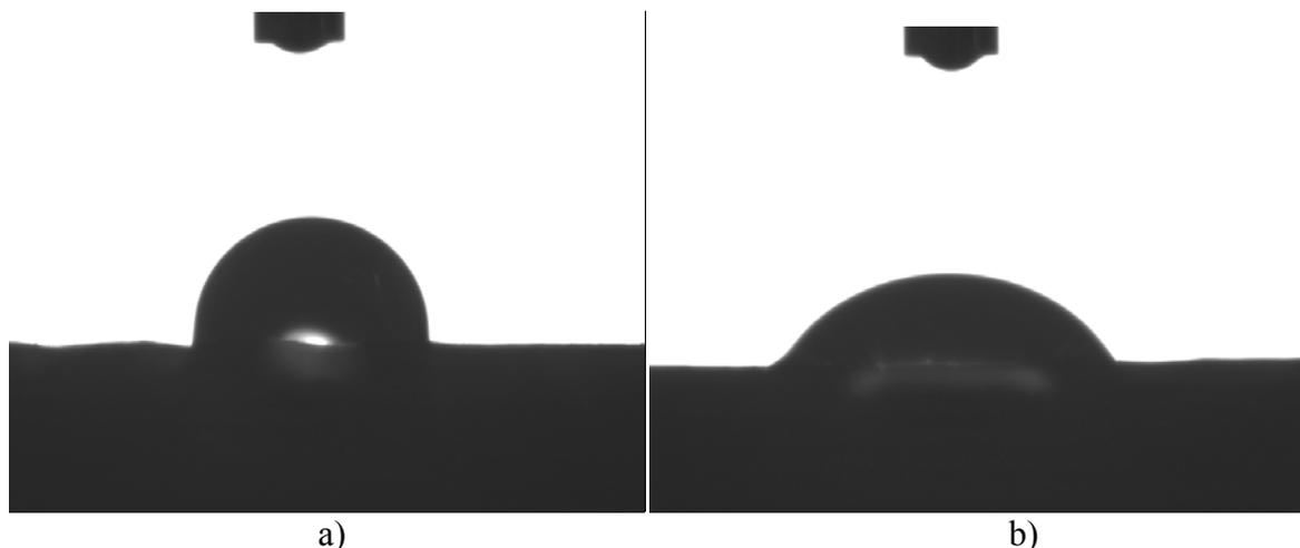
Fig. 1. Photographs of water droplets on the: a) laser non-modified and b) laser modified PCL sample surfaces
