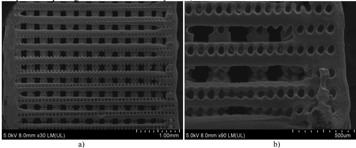
Fig. 2. a) General view of PCL sample after laser irradiation and b) with magnification
