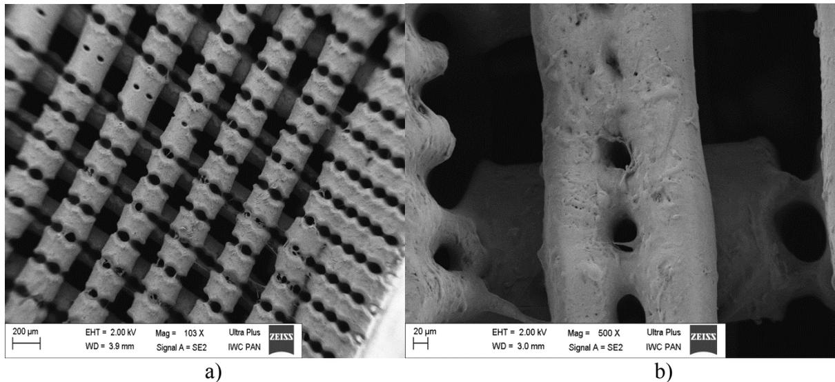
Fig. 4. SEM pictures of MG63 cells cultured for 7 days on the laser processed PCL sample, a) general view, b) single line from the sample
