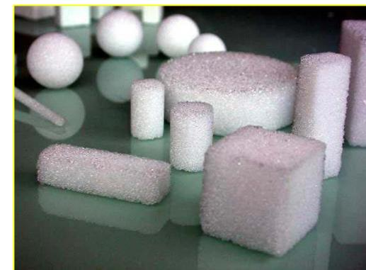
Impregnation of PMMA beads consolidated preforms with CaP powder suspension.
