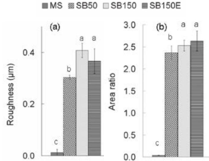
MS: mirror-polished, SB50: sand-blasted 50 μm
