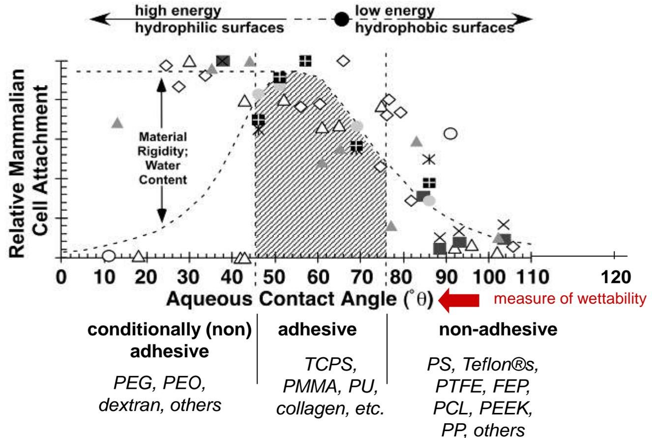
cells attach best to surfaces that are neither too hydrophobic or too hydrophilic
