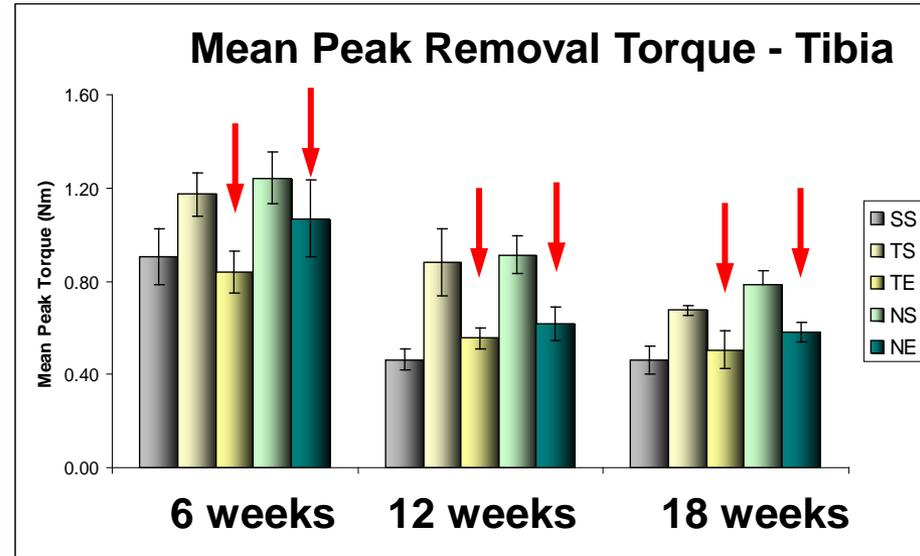
SS-polished stainless steel, TS-microrough Ti, NS-microrough TAN, TE-electropolished Ti, NE-electropolished TAN
