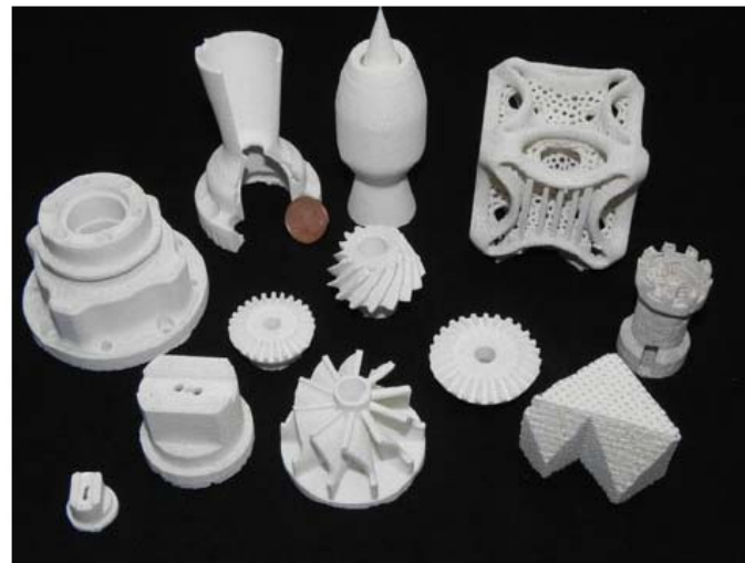
FIG. 15. Pure alumina parts processed by SLM.
