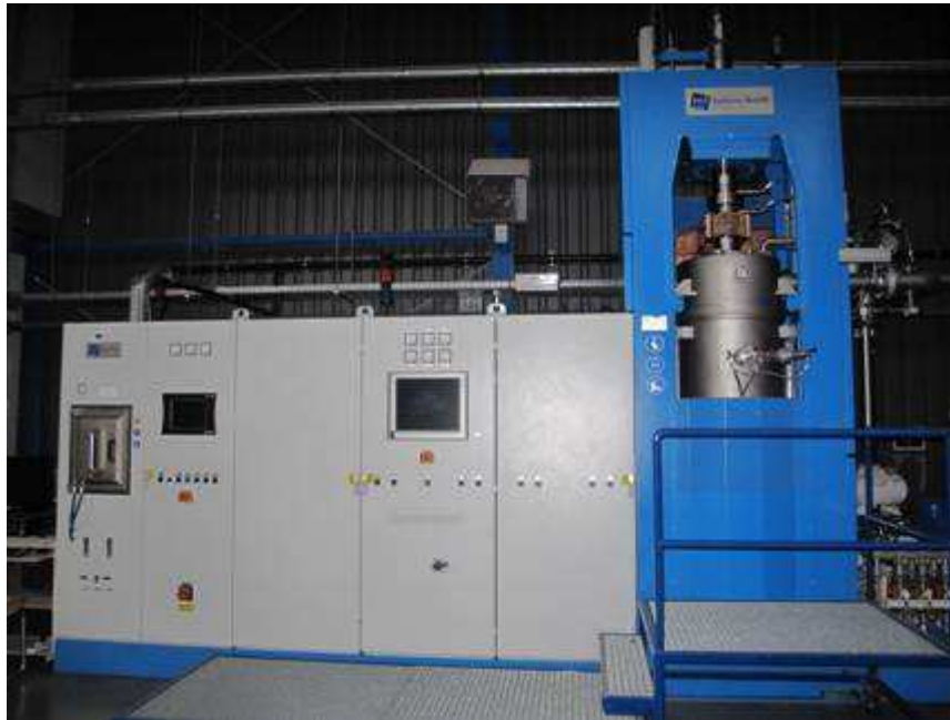
Spark Plasma Sintering From 25mm up to 160mm
