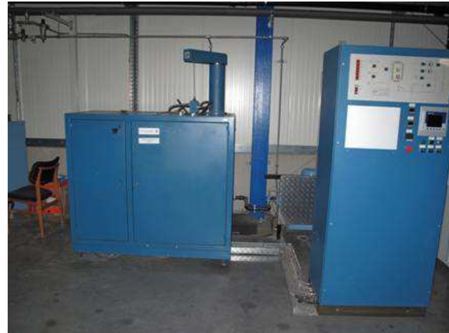
Hot Isostatic Pressing (under inert atmosphere, or up to 20% O 2 )
