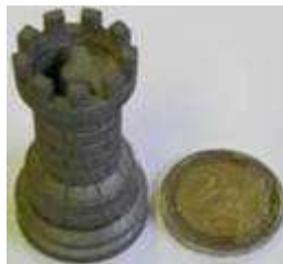
Selective Laser Sintering (Nd:YAG 200W)
