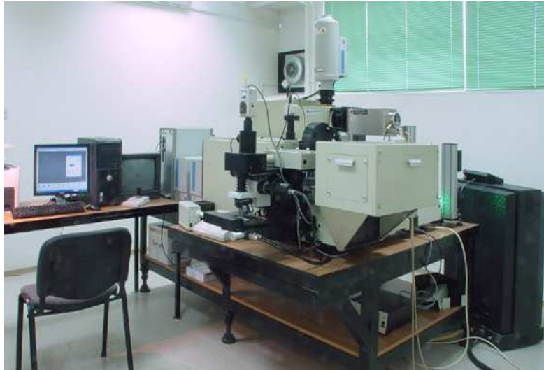
Raman spectrometer Horiba Jobin Yvon T64000
