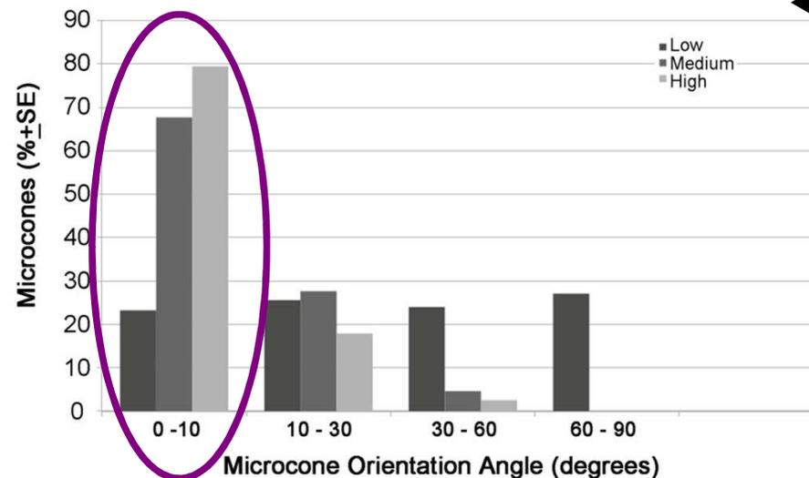
Whereas at the lower laser fluences the spikes don't seem to exhibit a preferred orientation, **as the laser fluence increases, the spikes present a striking parallel aligned orientation**
