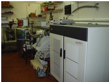
EPR spektrometer Bruker FT-EPR 580 Elexsys Continous wave and pulse mode 1- and 2-D measurements, temperature range 4-370K
