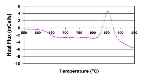
DSC trace for a BG optimised for viscous flow sintering. Note the large processing window between Tg and Tcon
