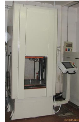
Pressure slip casting (PSC)
