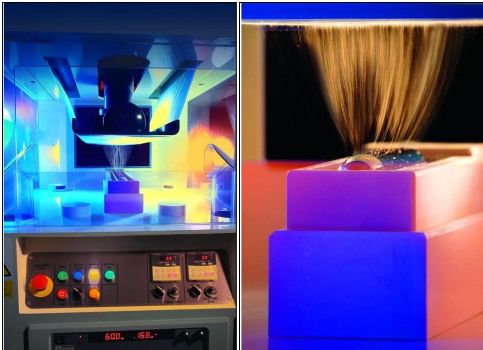
Photos (from www. Elmarco.com ) of electrospinning Nanospider TM equipment situated in KTU Department of Materials Engineering
